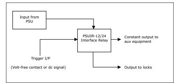
Fig 1: PSUIR - Typical System Design
