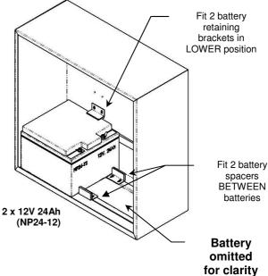
Risk of explosion if battery is replaced by an incorrect type.
