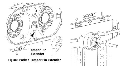
Fig 4b: Fitment of Tamper Pin Extender
