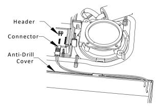
Fig 6: Connecting Anti-Drill Cover
