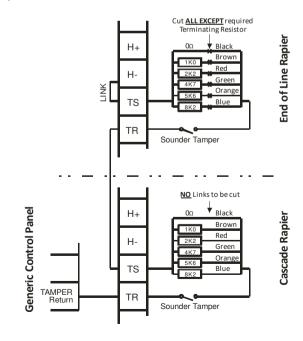
Fig 2: Multiple Cascade Rapier Tamper Connection
