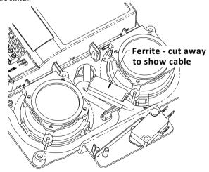
Fig 5: Fitting of Ferrite
