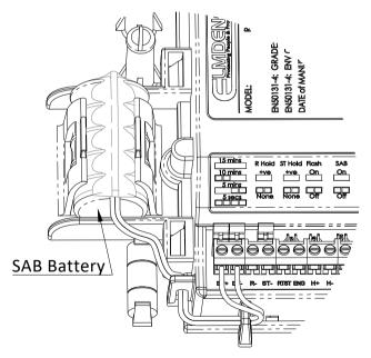
Fig 7: SAB Battery Removal and Replacement
