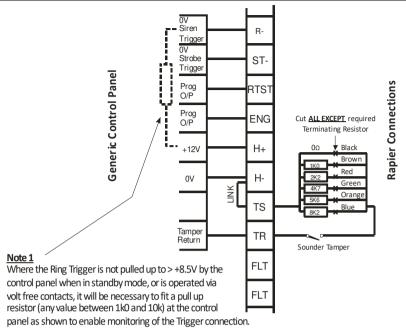
Fig 1: Single Rapier Tamper Connection
