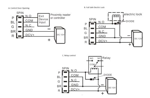
\*Connect diode when the control terminal is loaded, in order to absorb surge and prevent damage to sensor
