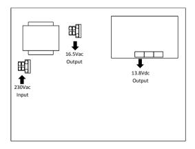
Fig.1 Power Connections
