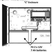
WARNING: ALWAYS FIT 2 BATTERIES and wire in series, the product will not work with a single 12V battery
