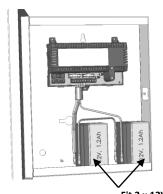
Fit 2 x 12V 1.2 Ah batteries
