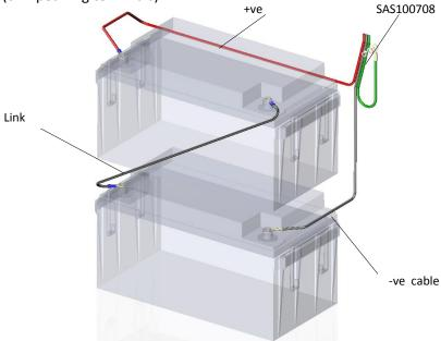
Route the positive (red lead) of the 3m cable to the positive terminal of the upper battery
