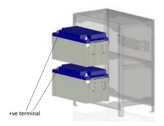
Fit positive and negative ends of 3m cable (SAS100709) to the batteries as shown (crimped ring terminals):
