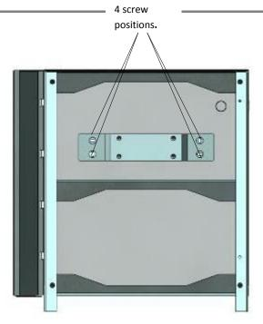
Position the case in its installation position. Spot through 4 fixing screw positions.
