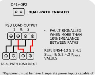
quipment must be have 2 separate power inputs capable o withstanding a short to ground on one path
