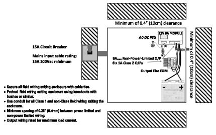
Fig. 1 Mounting of Power Supply
